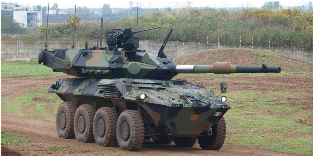
*On the ove with hatches closed and in the hunter-killer mode. The Centauro II can use all existing 120 mm ammunition. (Photo P. Valpolini)*
