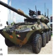
thermal sighting system with integrated laser rangefinder. The brand-new hull has a higher level of ballistic and mine protection. It is powered by an Iveco diesel developing 720hp, coupled to an ZF automatic transmission, which gives a maximum road speed of 105km/h.
